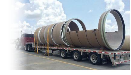
the streets above and reduces treatment costs. HOBAS pipe has a consistent, mold-smooth O.D. The pipes seal perfectly to molded and precise tolerance machined couplings.
