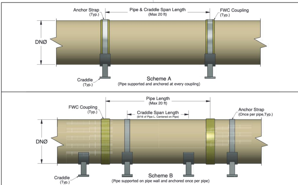
FIGURE 20 - Pipe Support Spacing and Scheme
