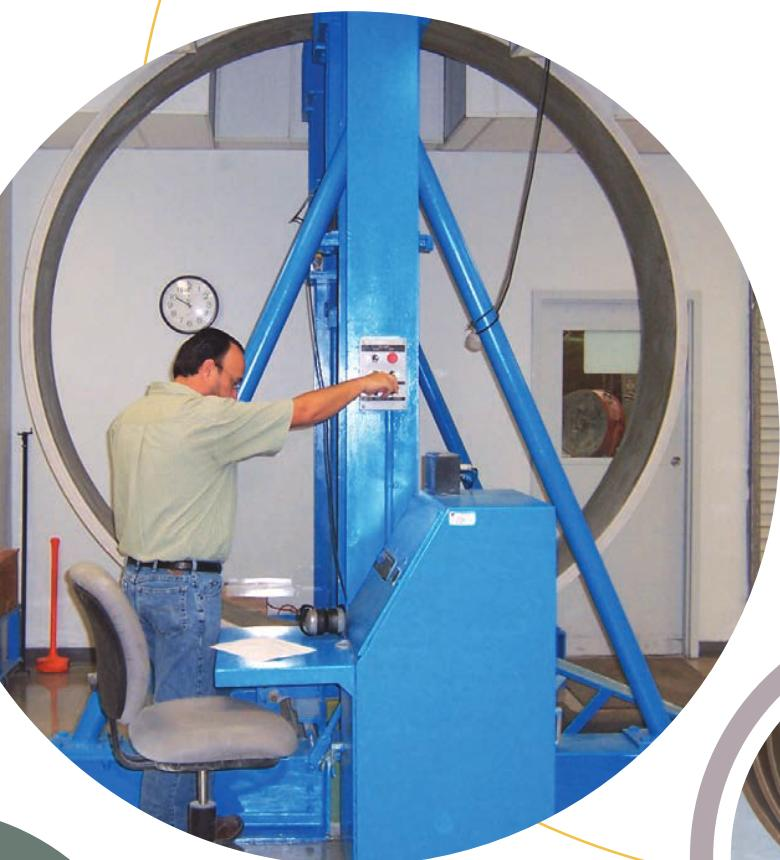
*Pipe stiffness is tested frequently to assure high performance.*
