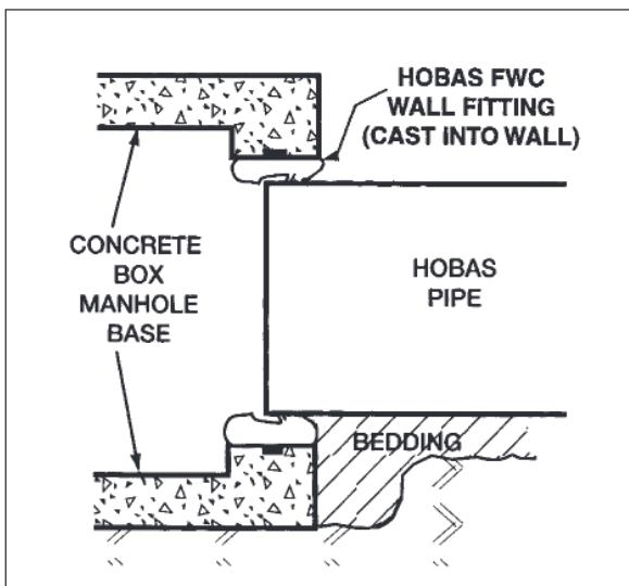
**FIGURE 8 - HOBAS FWC Wall Fitting Connection**
