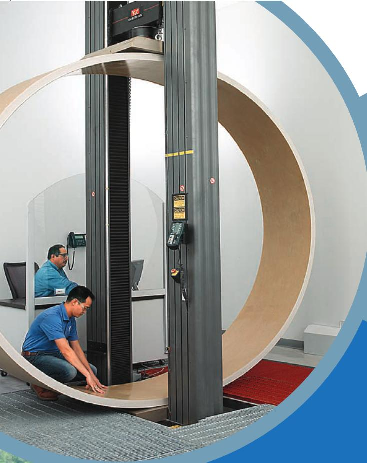
Every step of the HOBAS manufacturing process is carefully controlled and verified. In the Quality Control lab, samples taken from the production line are checked for adherence to the standards and specifications.
