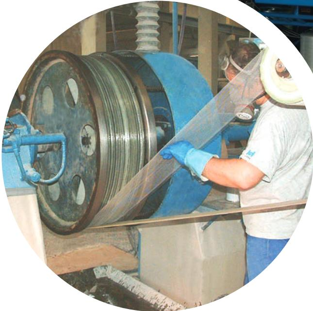
Pipe materials feeders are computer controlled. This helps assure consistent high quality. Multiple facilities around the world manufacture CCFRPM pipe using HOBAS technology.
