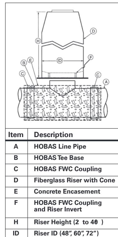
**FIGURE 4 – HOBAS Tee Base Manhole System with Riser & Cone**
