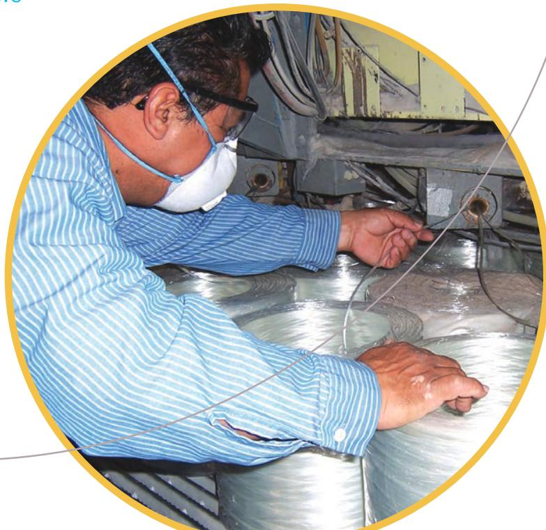
Fabrication of HOBAS FWC high strength coupling.
