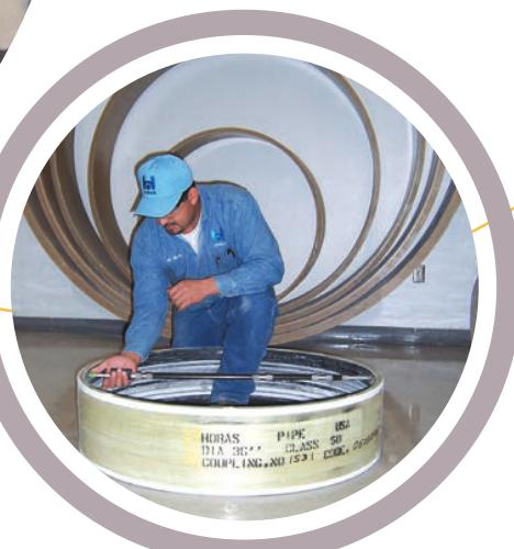
*All pipes and couplings are completely inspected.*
