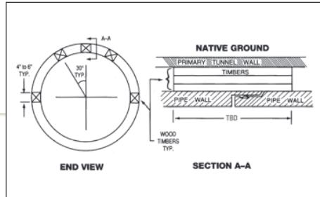
FIGURE 22 -Typical blocking scheme at each flush joint.
