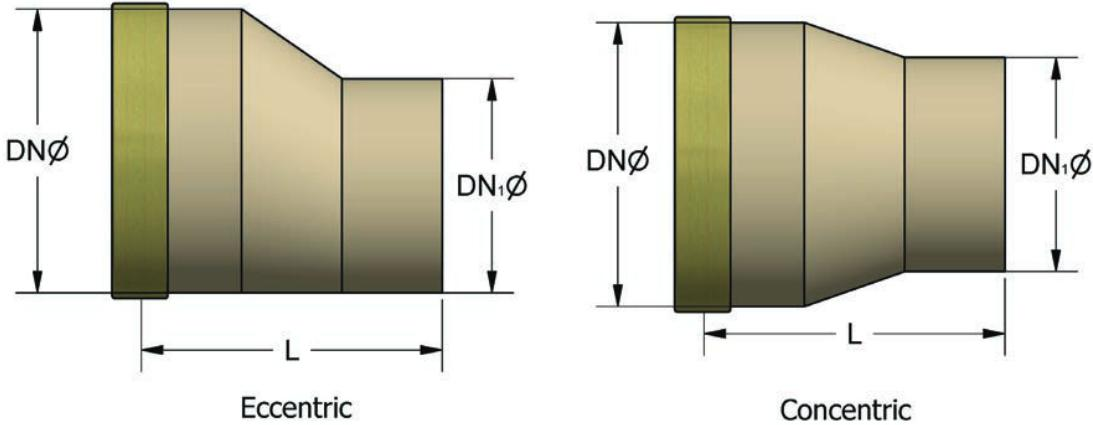
**Note:** Length of tapered portion is  $1.5 \times (\text{DN} - \text{DN}_1)$
