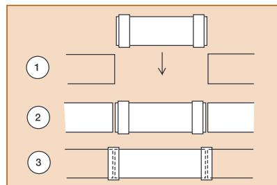
**FIGURE 2** - Closure coupling installation & assembly.
