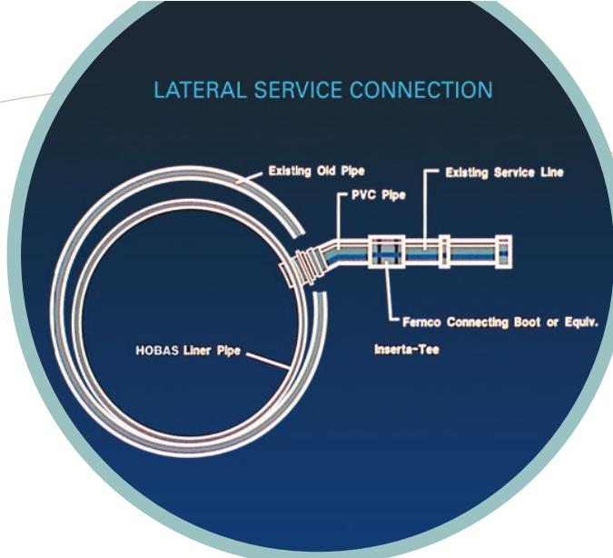
Lateral Service reconnection using an "Inserta Tee".
