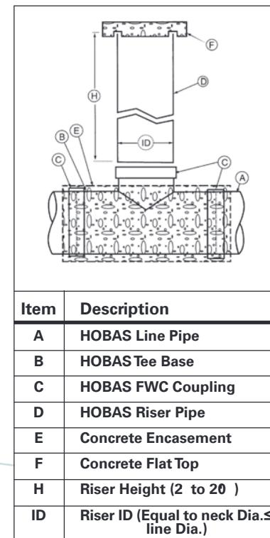
**FIGURE 5 – HOBAS Tee Base Manhole System with Riser & Flat Top**
