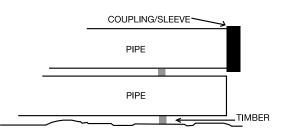
2. Always use timbers and chocks between layers when stacking pipe.
