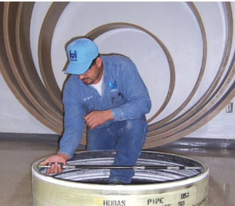
Each pipe and joint are monitored before leaving the plant.
